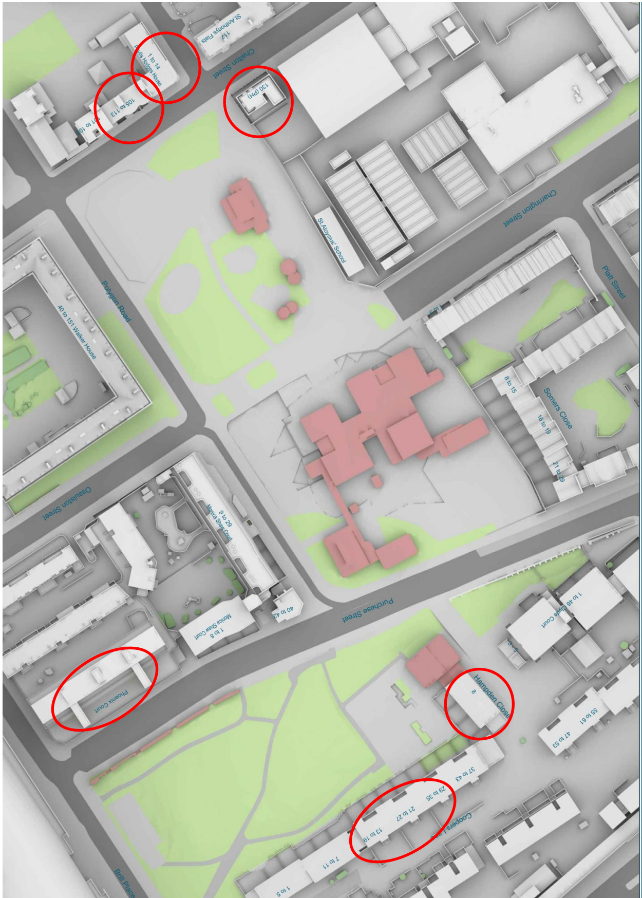
Figure 5 – Properties assessed in Daylight, Sunlight and Overshadowing Report, with the most affected properties circled in red
