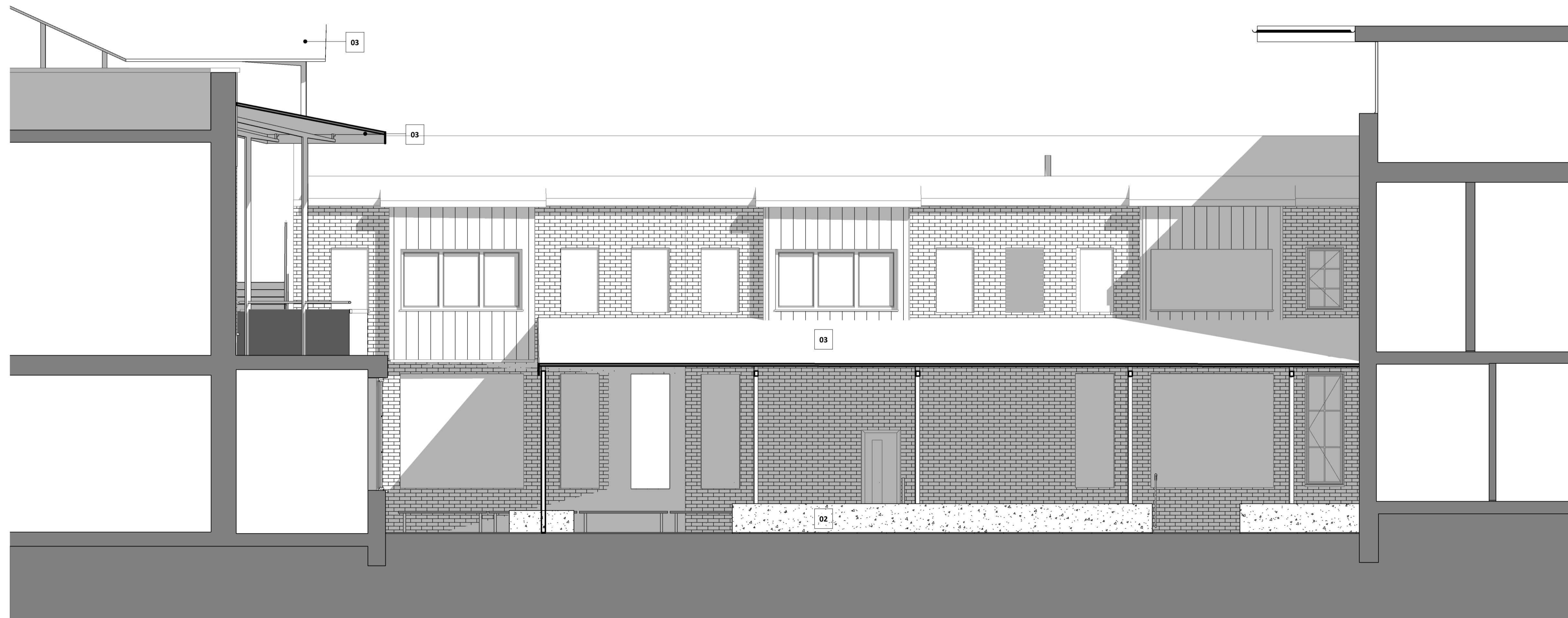
1. Proposed Courtyard South Elevation SCALE - 1 : 50@A1
