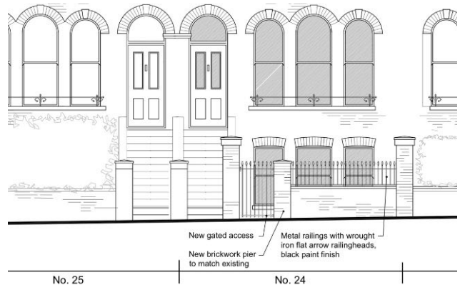
Proposed street boundary wall with new brick pier, gate access and railings.
