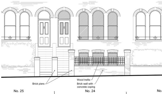
Existing street boundary wall with wooden trellis
