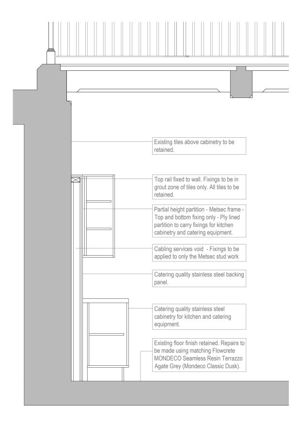
1 Proposed fixing of Catering equipment
