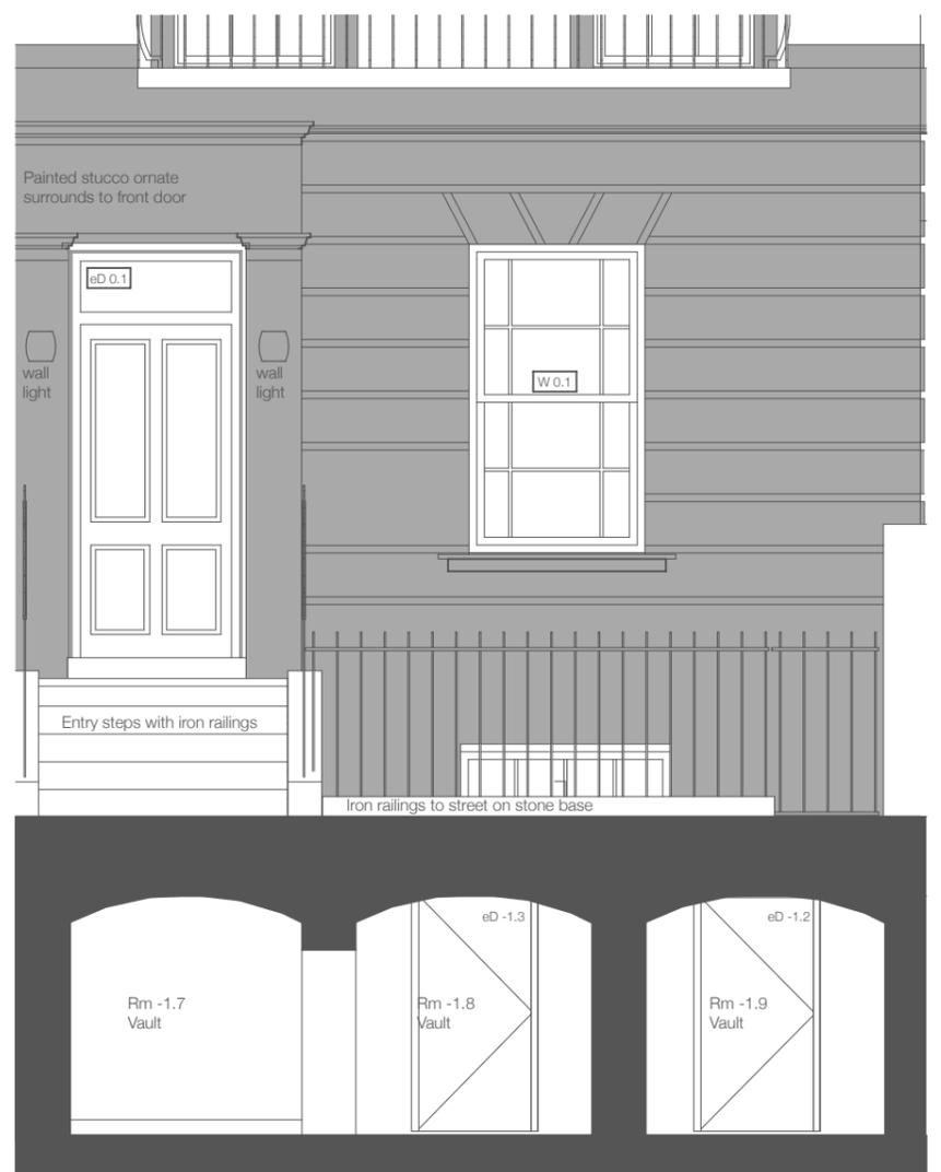
A.2 Front (South) elevation through street and vaults
