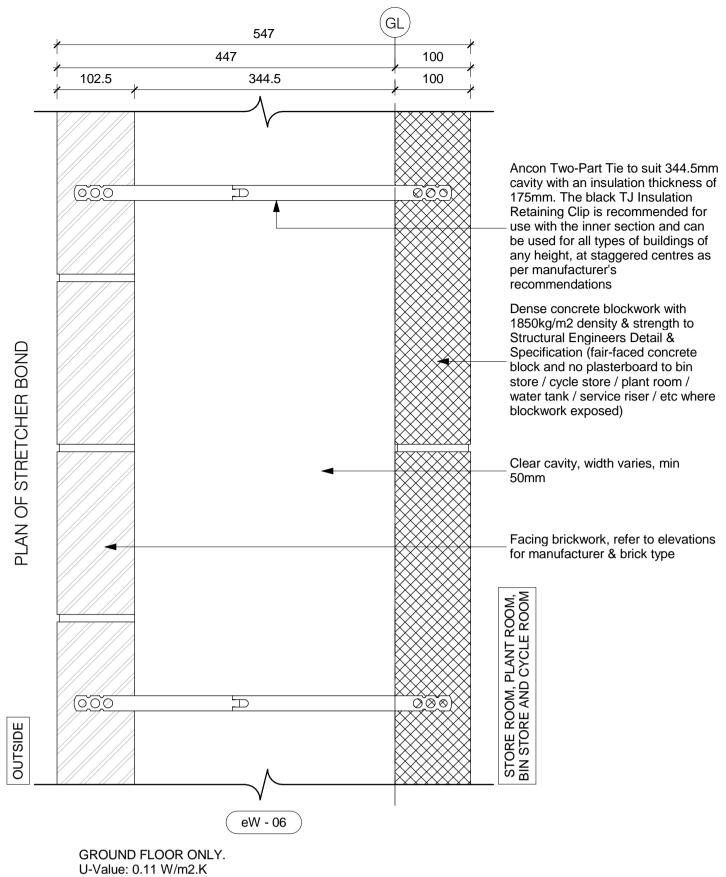
GROUND FLOOR O U-Value: 0.11 W/m2. Fire Rate: 2hrs min. Acoustic isolation: 5d
