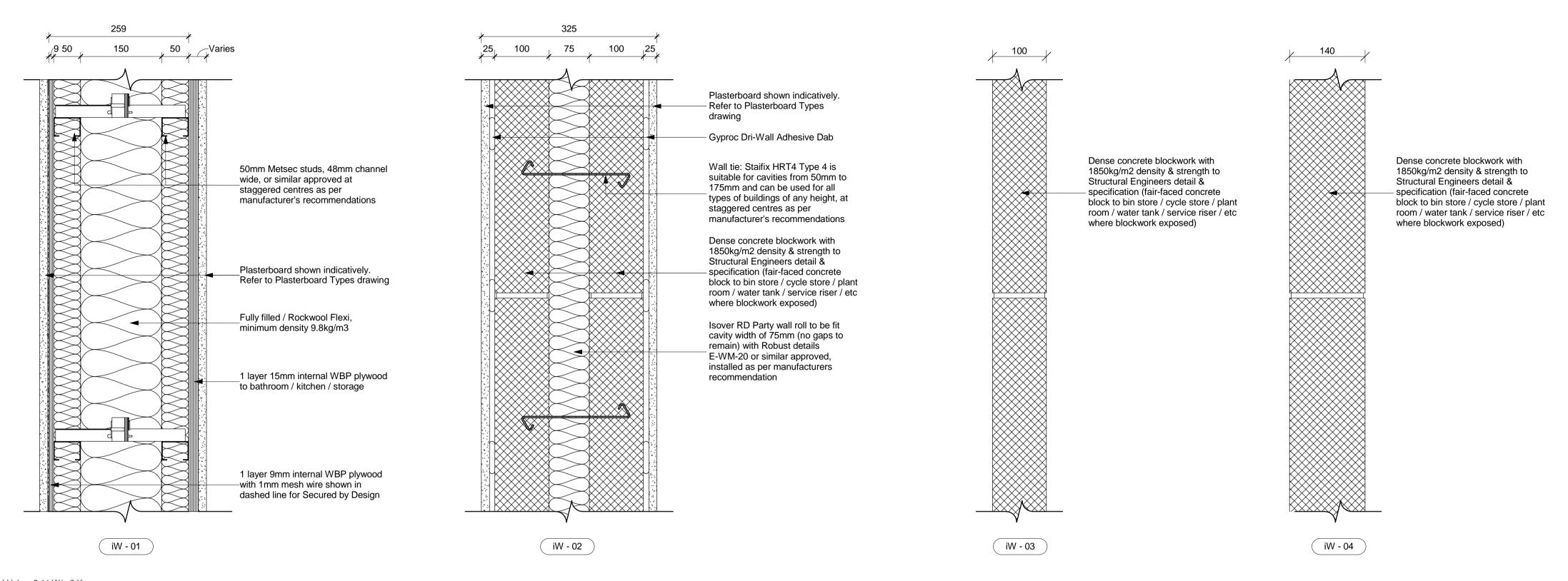
U-Value: 0.11 W/m2.K Fire Rate: 2hrs min. Acoustic isolation: Refer to Acoustic isolation requirement table at tight. All dimensions to be verified on site by Main Contractor before the start of any shop drawings or work whatsoever either on their own behalf or that of subcontractors.
