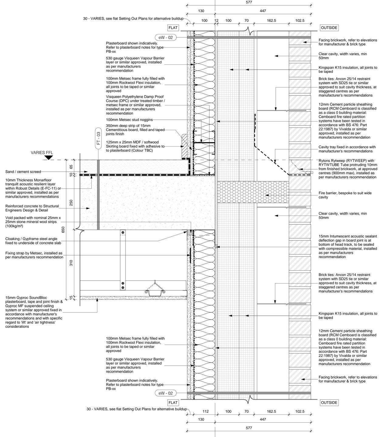
2 Typical Section of External Wall (Stretcher Bond) & Separating Floor between Flat to Flat
