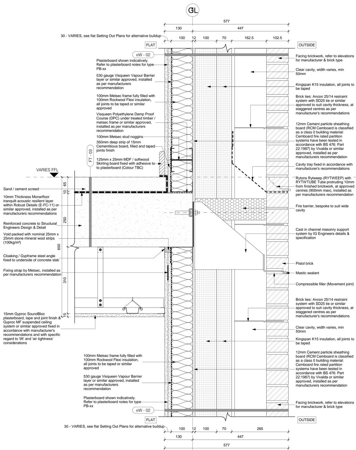
1 Typical Section of External Wall with Cast in channel masonry support system (Stretcher Bond) & Separating Floor between Flat to Flat
