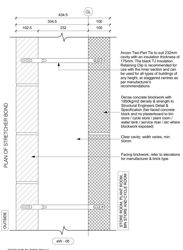
GROUND FLOOR ONLY. U-Value: 0.11 W/m2.K Fire Rate: 2hrs min. Acoustic isolation: 5dB improvement over building regulations minimum.
