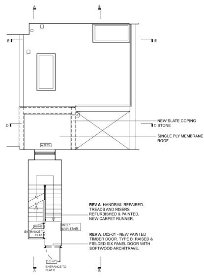
PROPOSED SECOND FLOOR PLAN DRAWN INCORRECTLY IN ORIGINAL PLANNING APPLICATION
