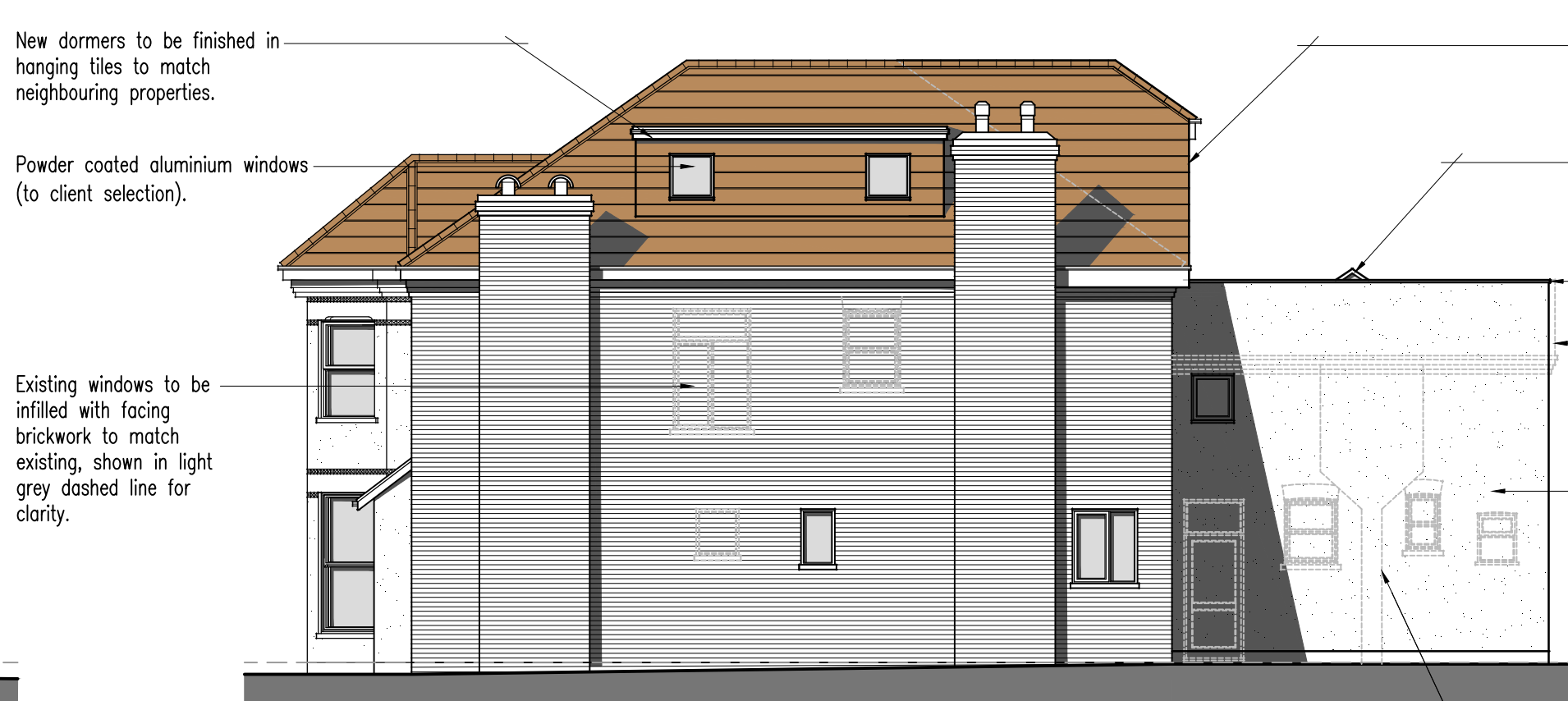
Proposed Side Elevation 1:100
