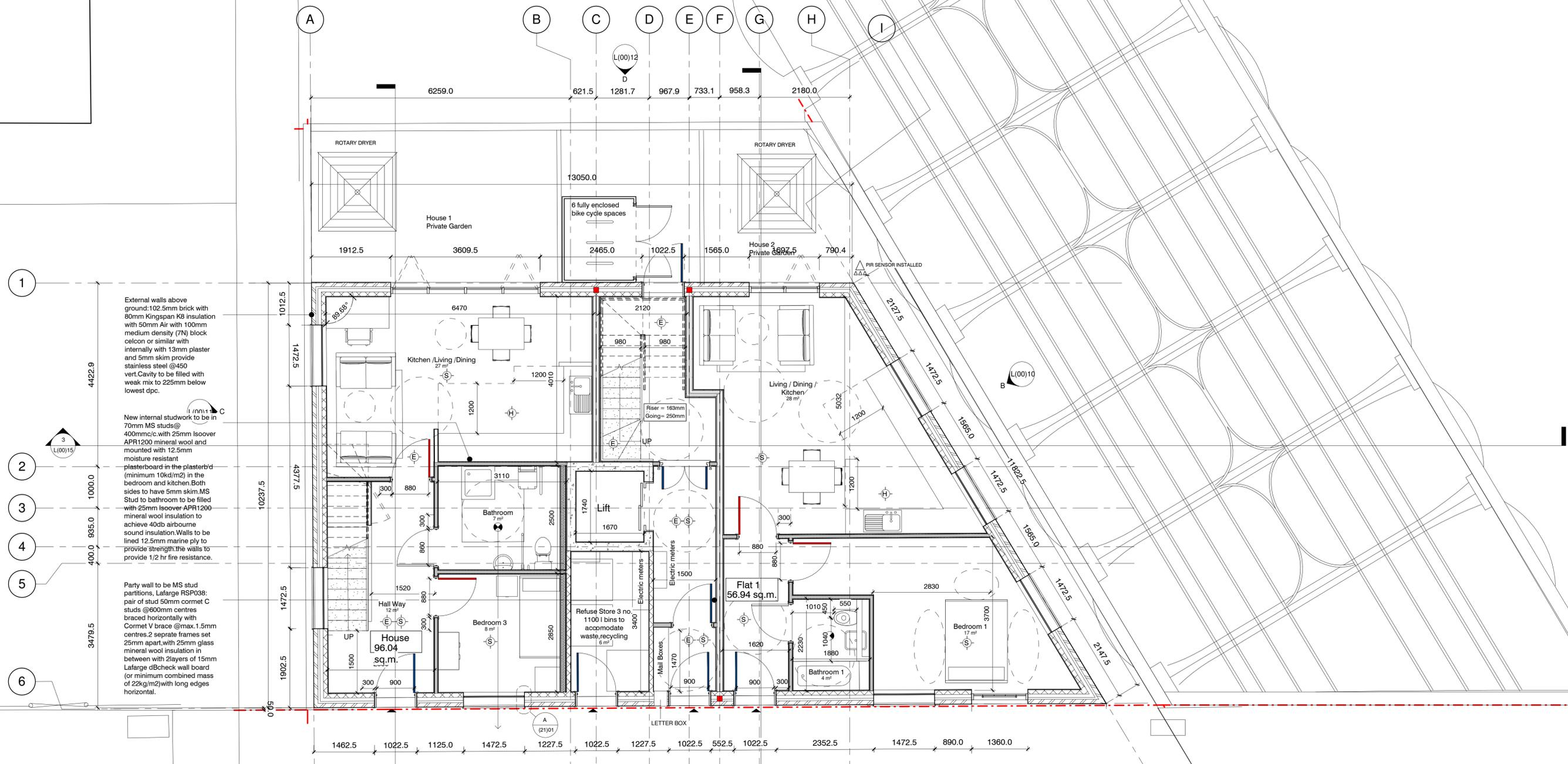
External walls above ground: 102.5mm brick with 80mm Kingspan K8 insulation with 50mm Air with 100mm medium density (7N) block calccon or similar with internally with 13mm plaster and 5mm skim provide stainless steel @450 vert. cavity to be filled with weak mix to 225mm below lowest dpc.
