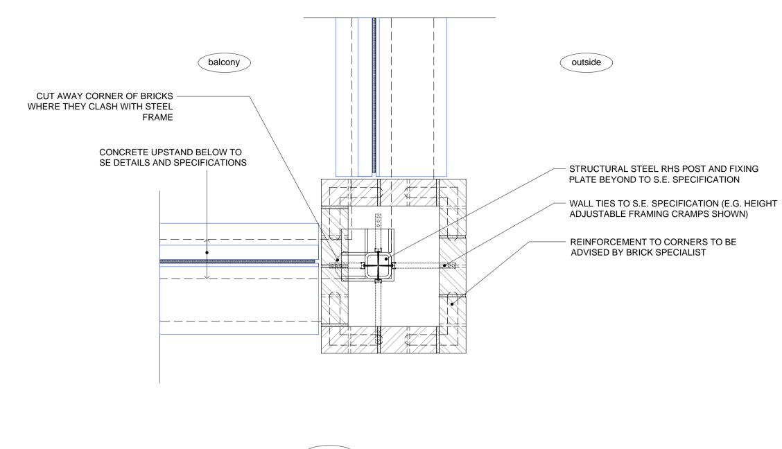
DETAIL - Block C - D-J-RC133 - Structural Post Encapsulation WT-RC1 (L03 to 07 GL E-09)
