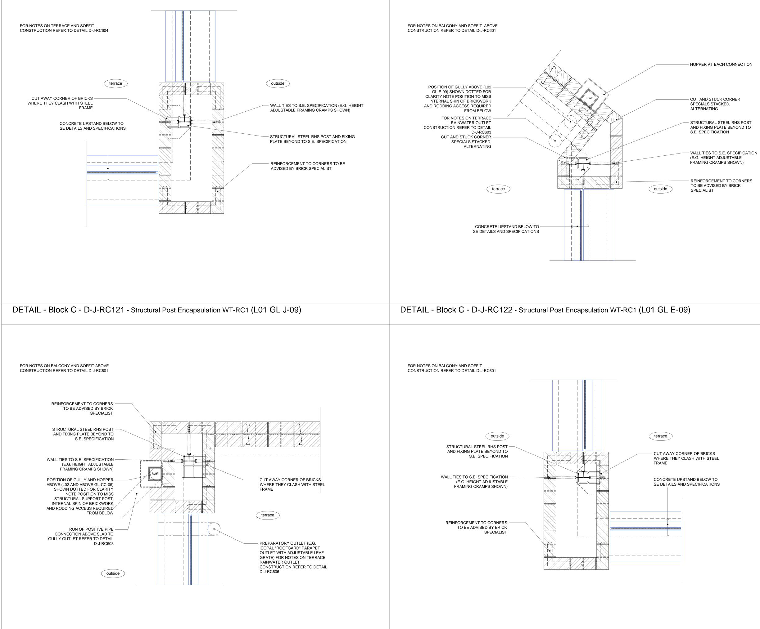
DETAIL - Block C - D-J-RC123 - Structural Post Encapsulation WT-RC1 (L01 GL CC-05)
