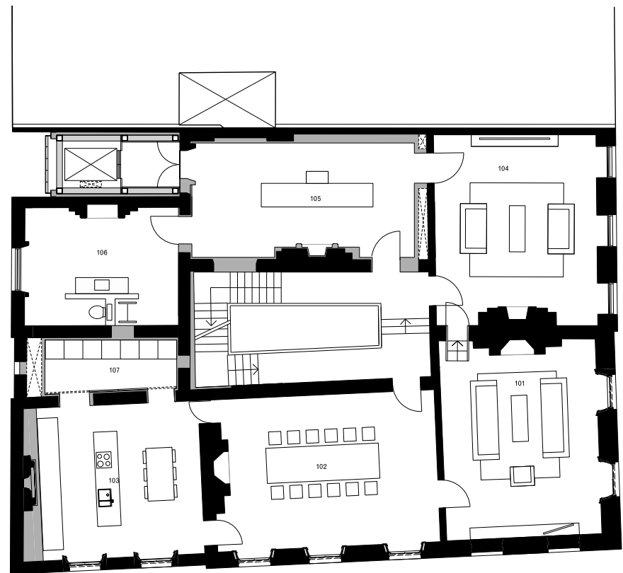
Figure 46: First Floor Plan (new work light grey) (©DCA).
