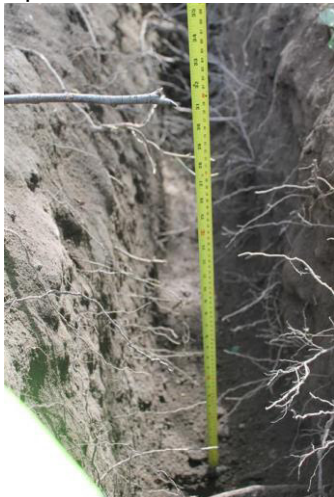
Photo 17. Depth of Trench 2 at 800mm.
