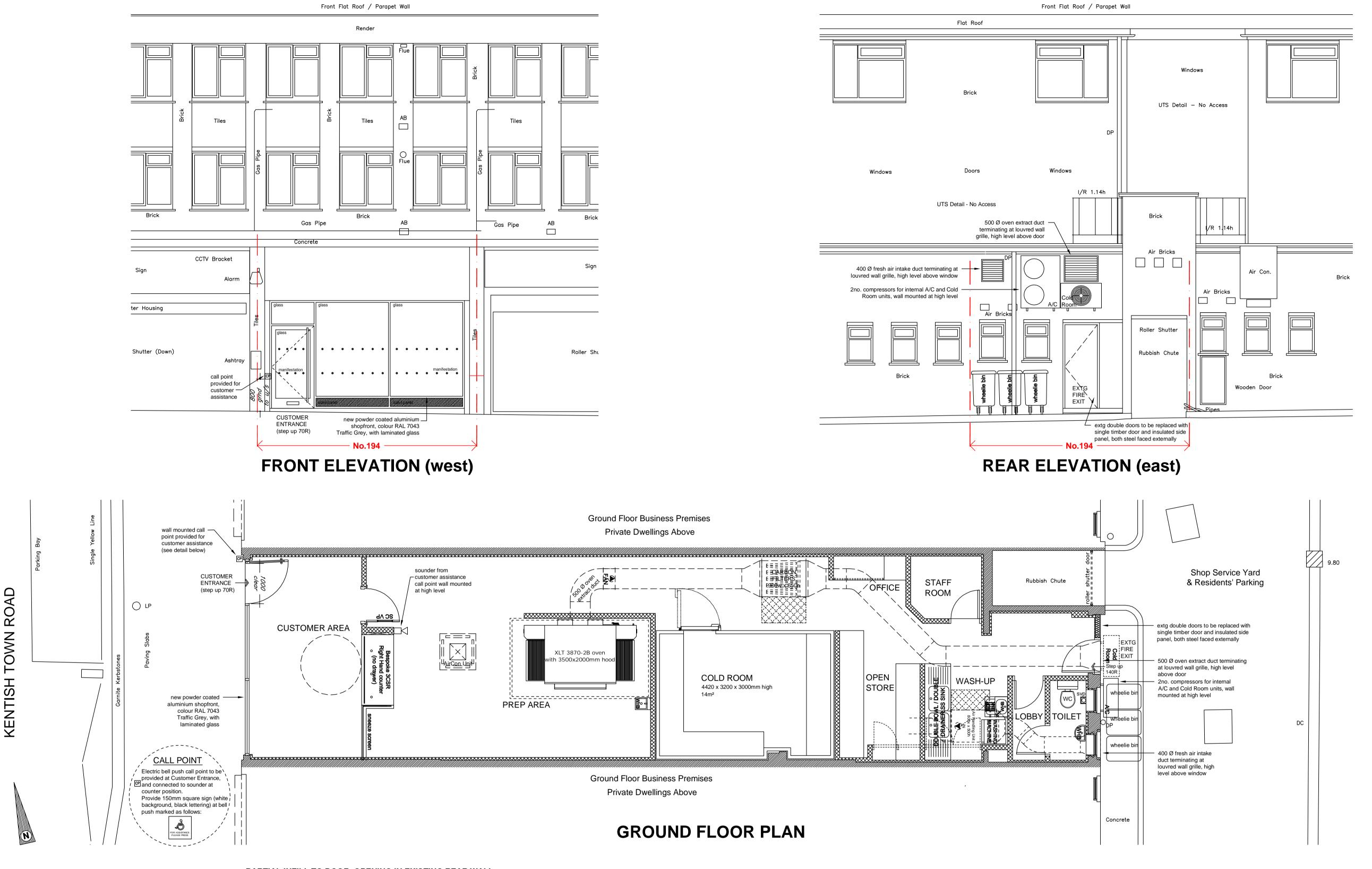
PARTIAL INFILL TO DOOR OPENING IN EXISTING REAR WALL: Existing double doors to be replaced with single timber door and insulated side panel, both steel faced externally
