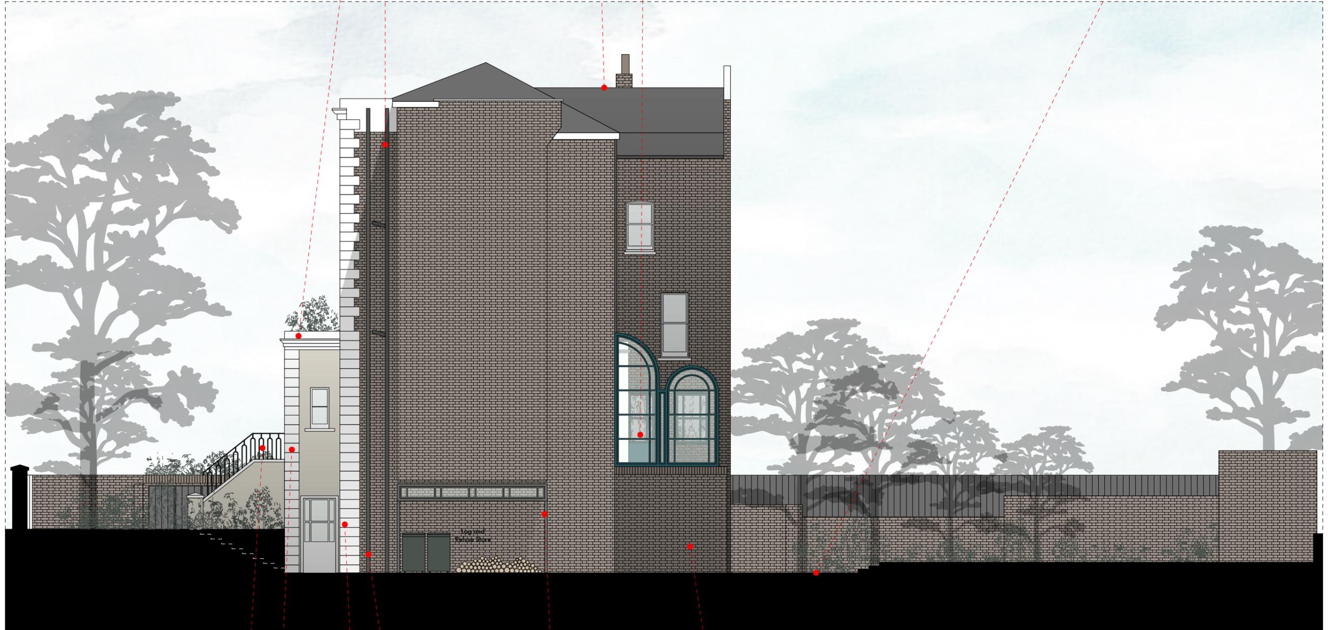
Roof cornice repainted, and flashing removed and planted behind parapet.
