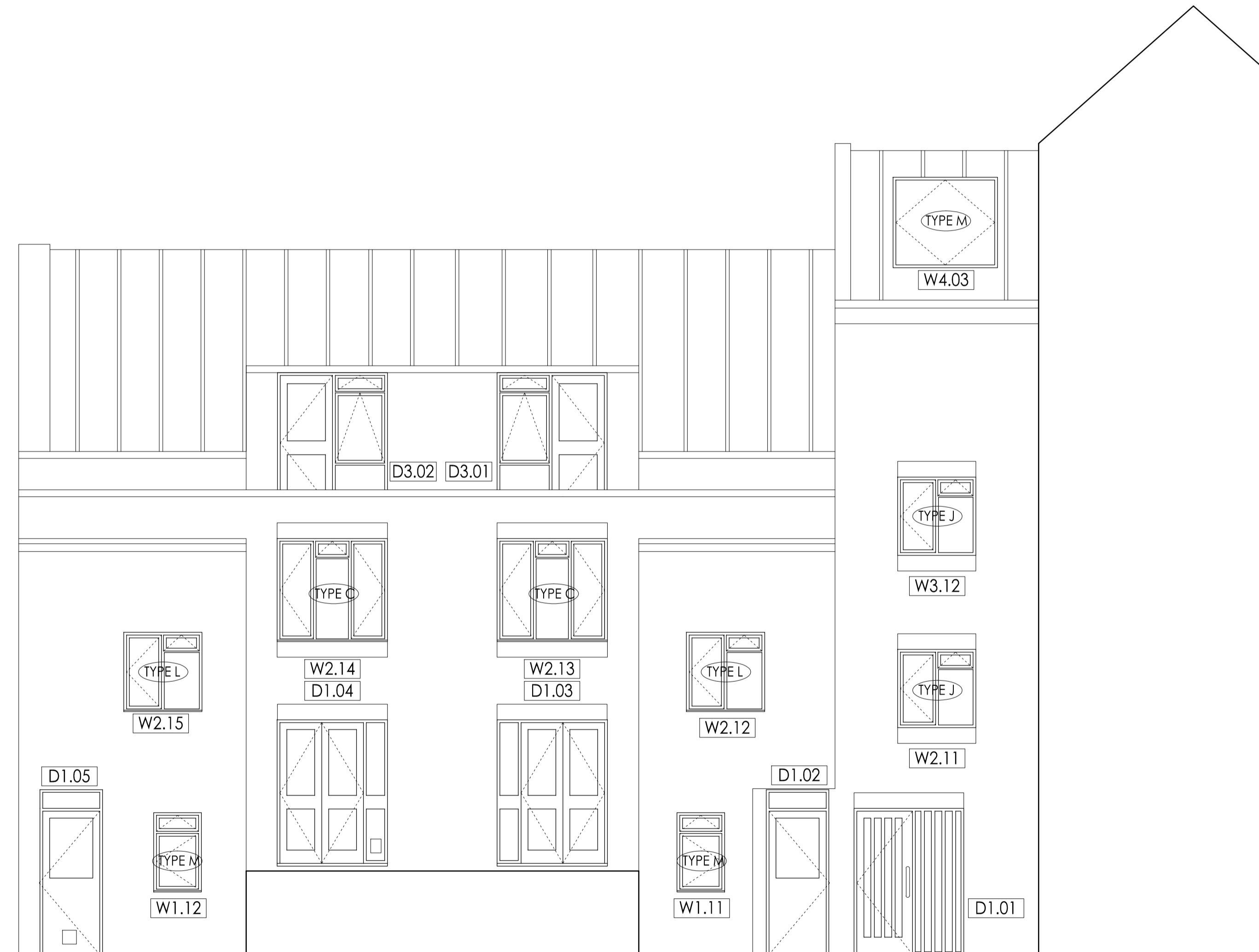
EXISTING ELEVATION D SCALE 1:50 @ A1
