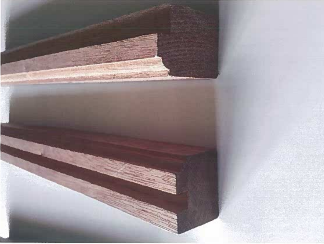
PHOTO 1 - Head and sash stile (right) and meeting rail (left) Profiles have been chosen to match the existing windows to the rear of the house.
