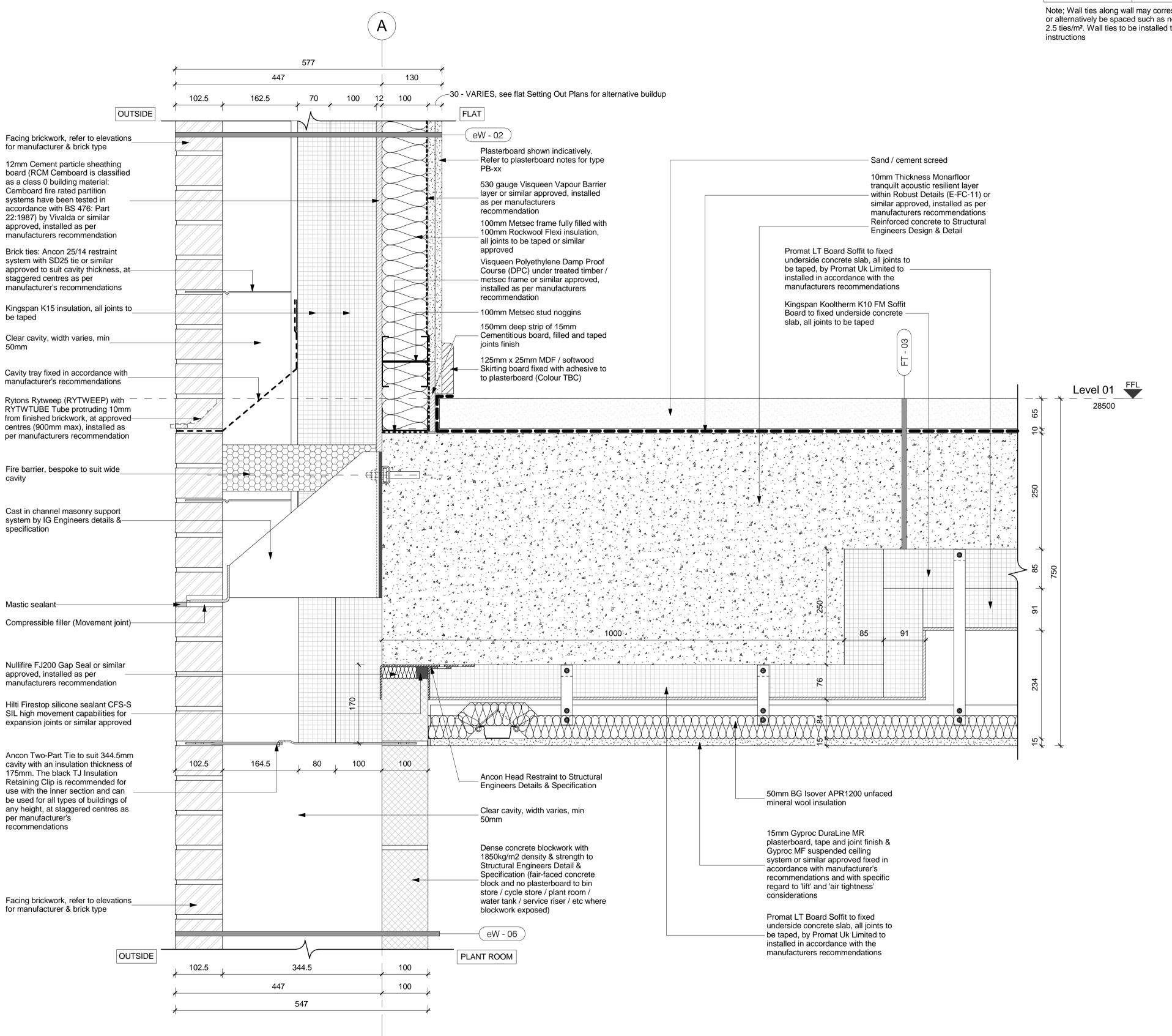
Section of External Wall with Cast in channel masonry support
