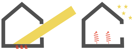
Examples of how the thermal mass absorbs heat during day and emits it during night.
