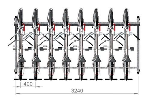
The TURVEC TUR8001 2ParkUp front fork support is designed to properly support a bicycle when parked on the gas assisted upper tier. The unique support ensures a bike is held in an upright position when parked and being loaded onto the top tier.
