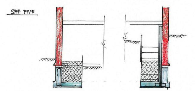
Repeat the above sequence for each underpinning bay, allowing a period of not less than two days between the dry packing of one bay and the excavation of adjoining bay.
