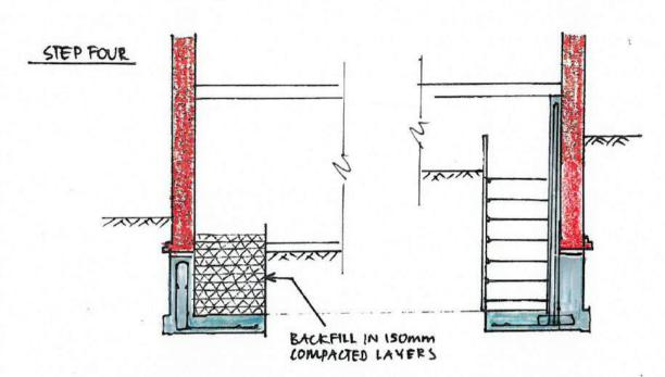
Following initial curing period of concrete (72 hours), pin up with semi dry sand cement mix between top of underpinning concrete and underside of existing foundation.
