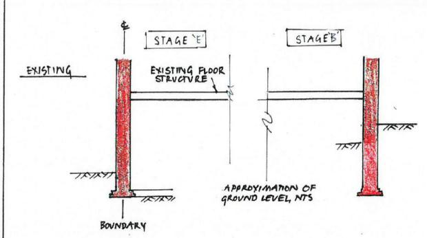
Sequence of underpinning to be 1,2,3,4,5 maximum bay length to be 1.0m. Excavate access trench and initial heading for the first pin. Check the condition of the existing brickwork and foundation. If badly damaged, cracked or loose footings are encountered, provide temporary propping to the underside of the footing to ensure that the structure above the underpinning bay is fully supported as the excavation of the underpinning heading proceeds.
