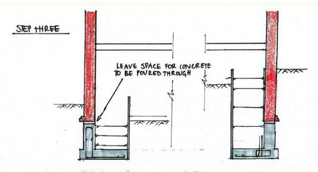
· Fill underpinning bay excavation with concrete to within 100mm of the underside of the existing foundation.
