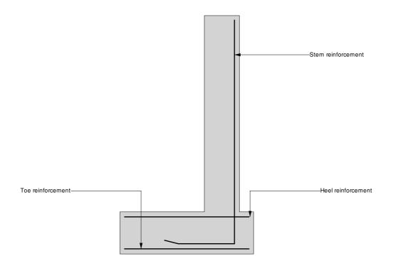
Toe bars - 12 mm dia.@ 200 mm centres -  $(565 \text{ mm}^2/\text{m})$ The design of the retaining wall heel is beyond the scope of this calculation! Stem bars - 12 mm dia.@ 200 mm centres -  $(565 \text{ mm}^2/\text{m})$
