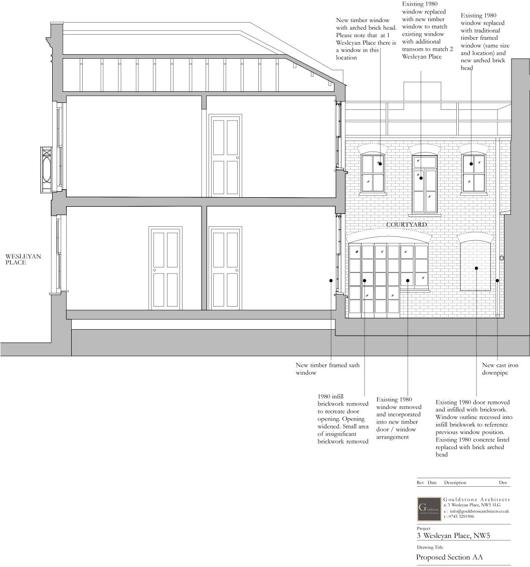
Scale 1:50 a3 Sheet **PLANNING** NOT FOR CONSTRUCTION Drawing Number 107\_PL1-GA04 Rev A Date 17.05.2016 Notes: Do not scale, use figured dimensions only. All dimensions must be checked on site. Inform the Architect of any discrepancies prior to construction. Please cross reference this drawing with all related Architect's, Engineers drawings and other relevant information Copyright (c) 2015 Gouldstone Architects. All rights reserved
