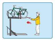
4. Lift the rack back into the horizontal position
