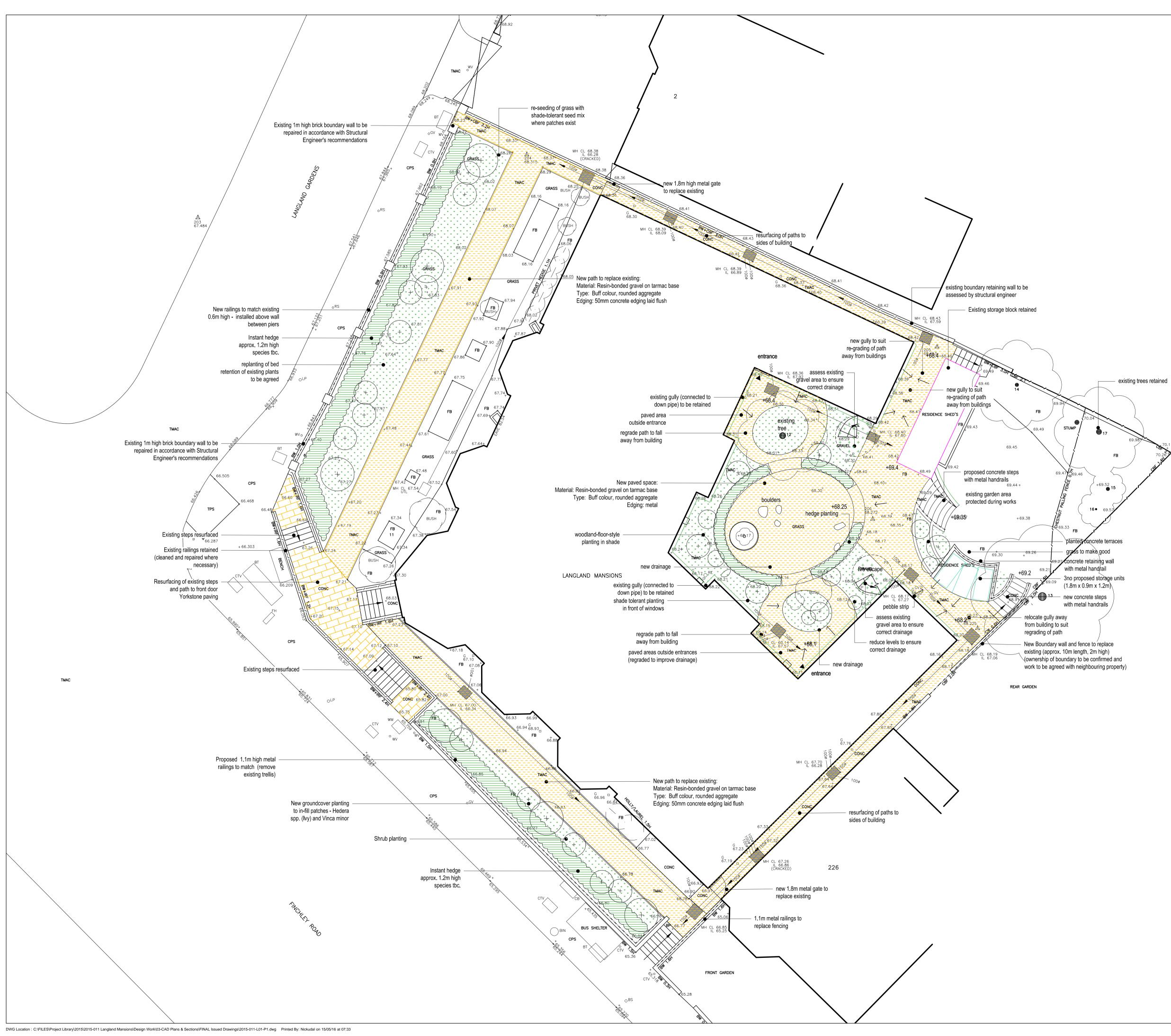
Key New Path to replace existing: Resin-bonded gravel finish Resurfacing to front entrance Yorkstone slabs Pebble surfacing + + + + + + for drainage Concrete edging to paths at front 50mm wide Curved metal edging to paving in back garden Proposed shrub planting ( + Proposed hedge planting Proposed re-planting Proposed metal railings/handrail \_.\_.\_
