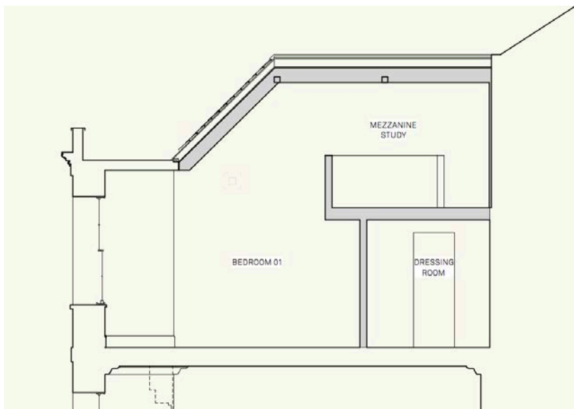
fig.15 Extract from proposed first floor & mezzanine section.
