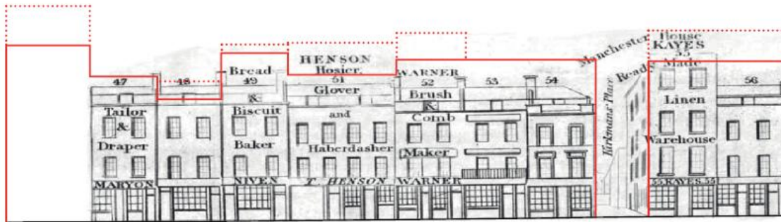
Fig: 3.4 John Tallis Elevation of Tottenham Court Road 1838-40 - Red line indicates building parapet heights; dotted line indicates mansard roof heights - Proposed nos. 51 - 52
