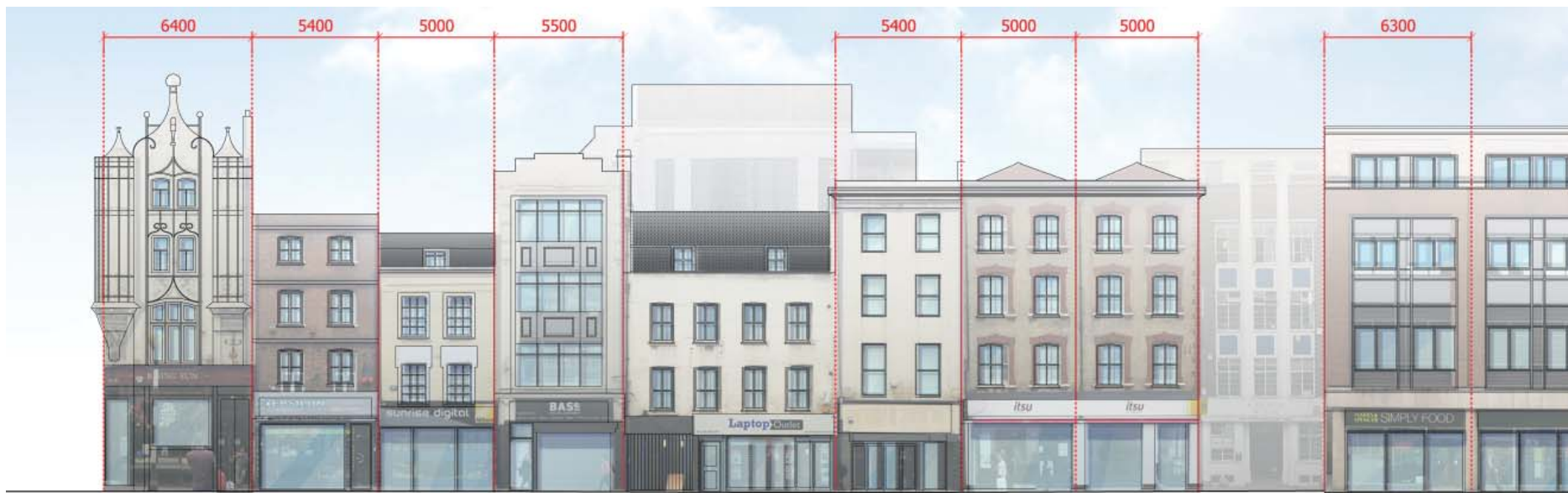
Fig: 3.14 Public (Front) Elevation - Urban grain clearly represented through varying ploth widths along street
