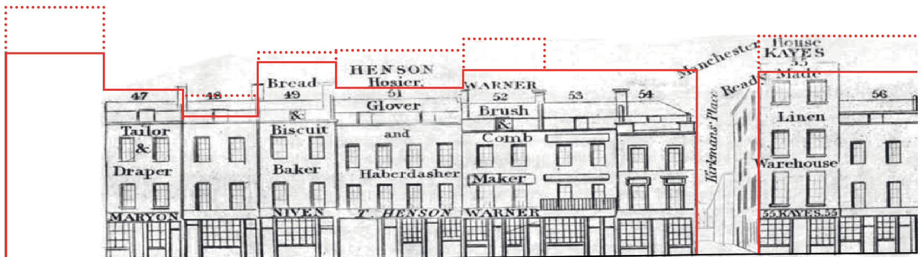
Fig: 3.4 John Tallis Elevation of Tottenham Court Road 1838-40 - Red line indicates building parapet heights; dotted line indicates mansard roof heights - Proposed nos. 51 - 52
