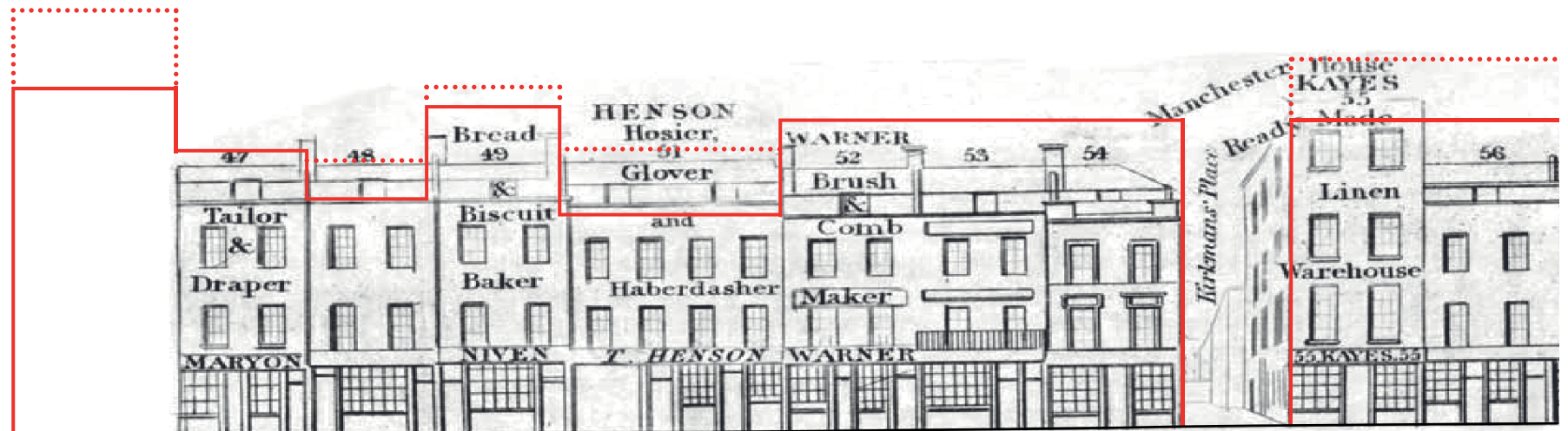
Fig: 3.3 John Tallis Elevation of Tottenham Court Road 1838-40 - Red line indicates building parapet heights; dotted line indicates mansard roof heights - Present / Existing
