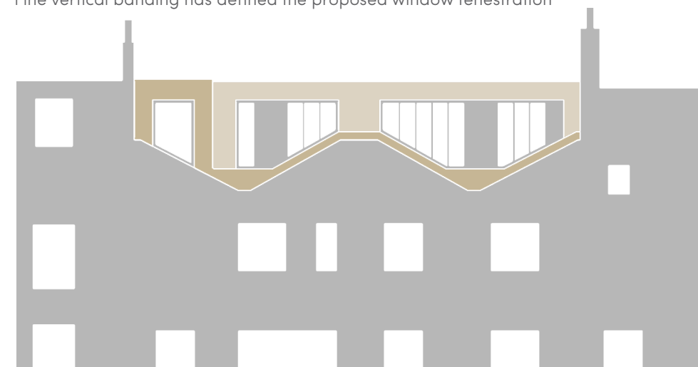
A band mimicking the butterfly parapet creates a transition between the existing and proposed. Also harmonising the materials of the existing elevation
