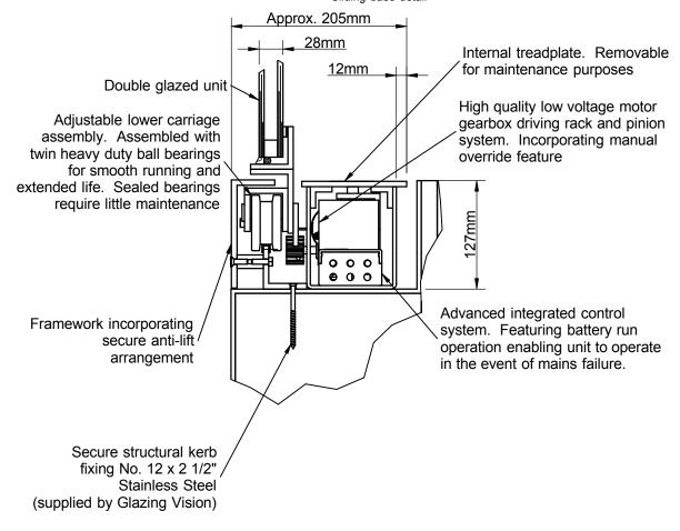
packers (supplied by Factory applied neutral Glazing Vision) cure low modulus silicone (standard = matt black) Approx. 260mm Factory applied structural glazing tape Powder coated aluminium framework standard colour RAL7015 slate grey. Factory applied 25mm brush draft seal Hard anodised track
