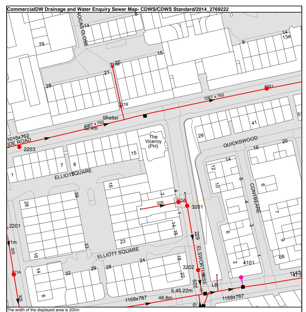
The position of the apparatus shown on this plan is given without obligation and warranty, and the accuracy cannot be guaranteed. Service pipes are not shown but their presence should be anticipated. No liability of any kind whatsoever is accepted by Thames Water for any error or omission. The actual position of mains and services must be verified and established on site before any works are undertaken.
