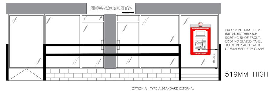
MILL LANE PROPOSED ELEVATION @1:50 OPTION A - TYPE A STANDARD EXTERNAL ATM PM PREFERRED OPTION NOTE: REQUIRES RECONFIGURATION OF STORE ¢ STRUCTURAL SURVEY IS NEEDED, DUE TO A BASEMENT AT THE PROPERTY
