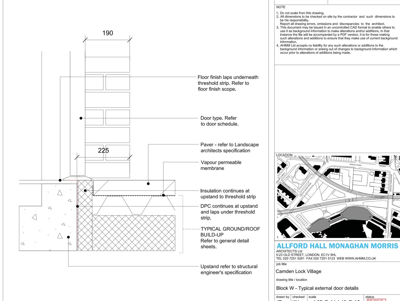
06 Base detail - Typical level threshold
