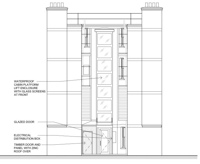
REAR ELEVATION SCALE 1:100 @ A3 BRF-P-300
