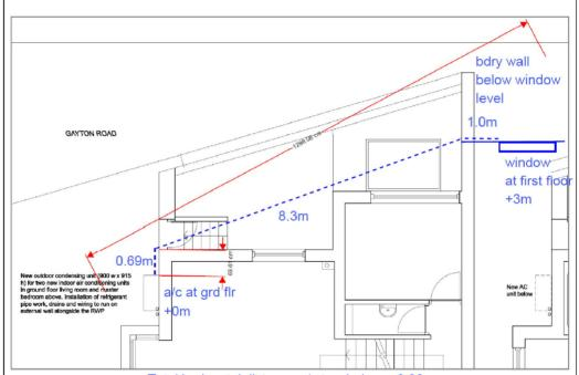
Total horizontal distance a/c to window = 9.99m Vertical distance a/c to window = 3m Total distance by shortest direct line = 10.43m
