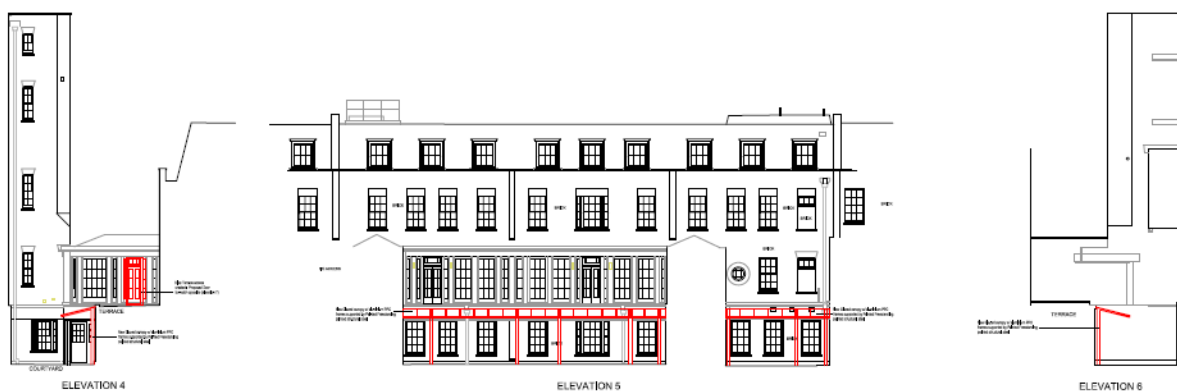
Internal Courtyard elevations – modifications shown in red
