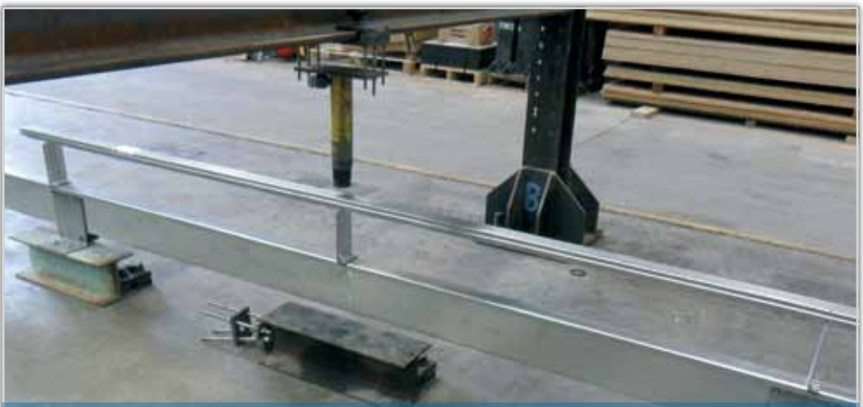
Matrix Spacer System undergoing testing at CERAM
