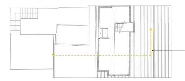
GAS PIPE FOLLOWS EXISTING RAINWATER PIPE ROUTE - AND DROPS TO KITCHEN FROM ABOVE. ALL VOIDS TO BE VENTILATED AS NECESSARY
