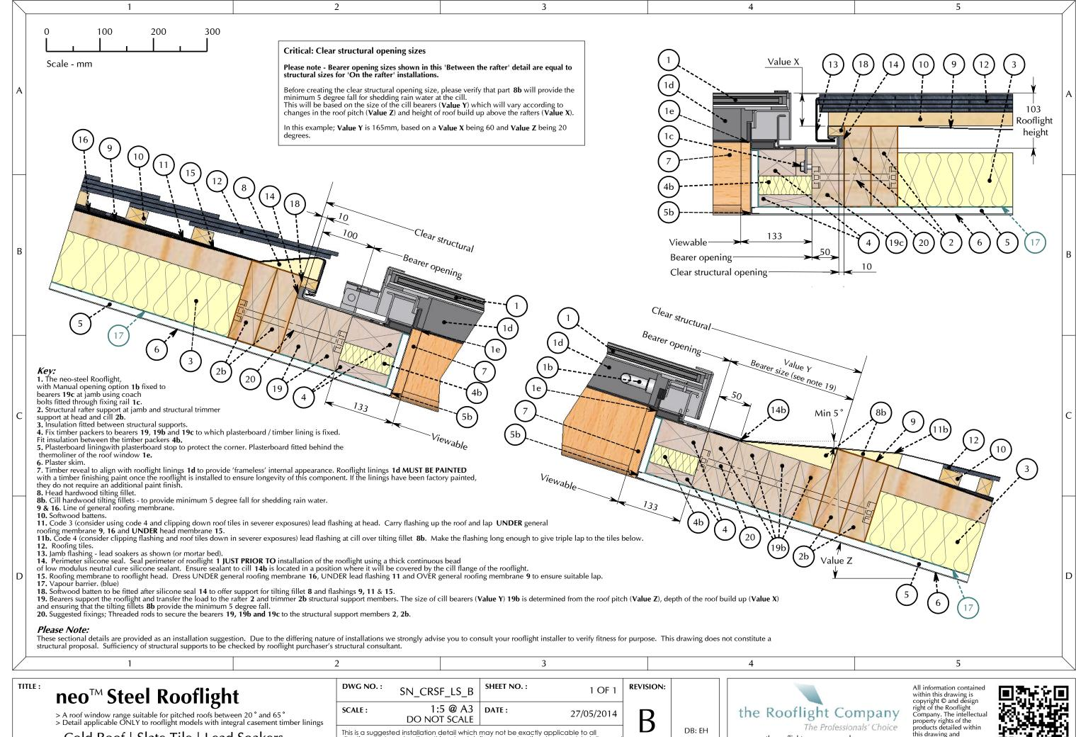
Cold Roof | Slate Tile | Lead Soakers 'Between the rafter' installation detail This is a suggested installation detail which may not be exactly applicable to all situations and constructions. It is not a detailed or constructional proposal. Installers and designers are advised to check their own details for compliance with all currently applicable Local Authority by-laws, Acts of Parliament and British / ISO standards
