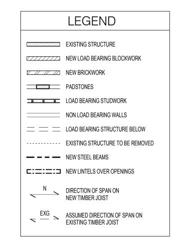
This drawing is to be read in conjunction with all relevant architects, engineers and specialists drawings and specifications.
