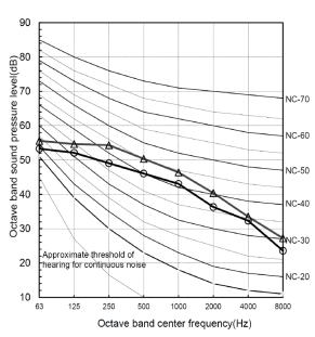
Noise data is in terms of overall dBA and linear dB free field sound pressure levels at 1m from the unit (per unit)
