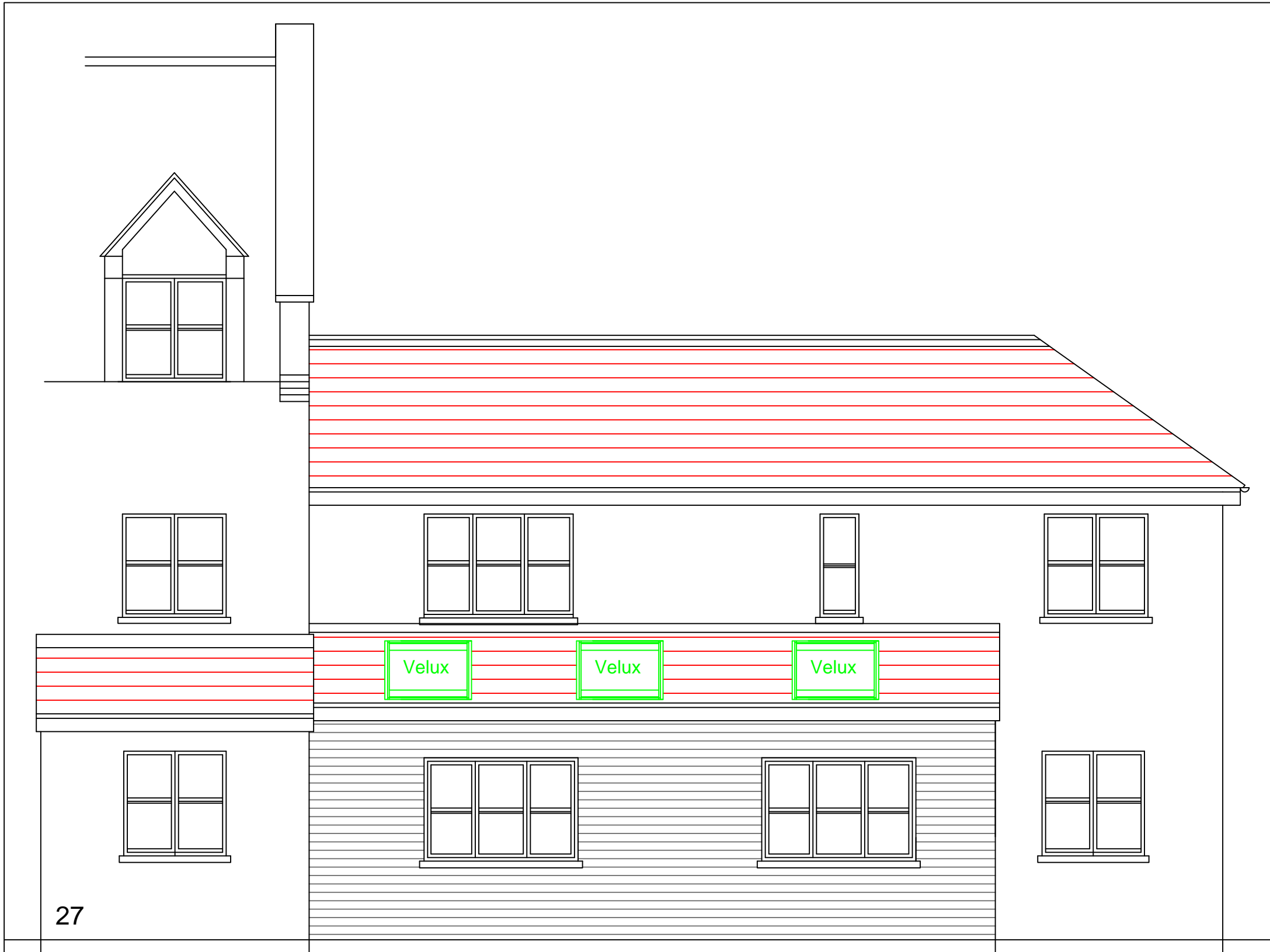
Rear extension in matching facing brickwork and bond with pitched tiled roof and Velux roof windows & matching rear facing casement windows PROPOSED REAR ELEVATION
