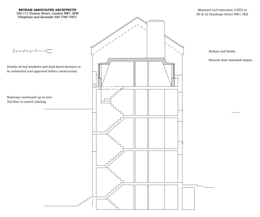
Scale @A4 1:100 Section: Proposed Drawing No 1205/19/a
