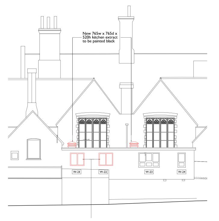
W21 and W22 - Existing louvred windows with metal grill surrounds to be removed. New painted external softwood framed double glazed windows with integral fly screen mesh to be installed to match adjacent Hall Store windows
