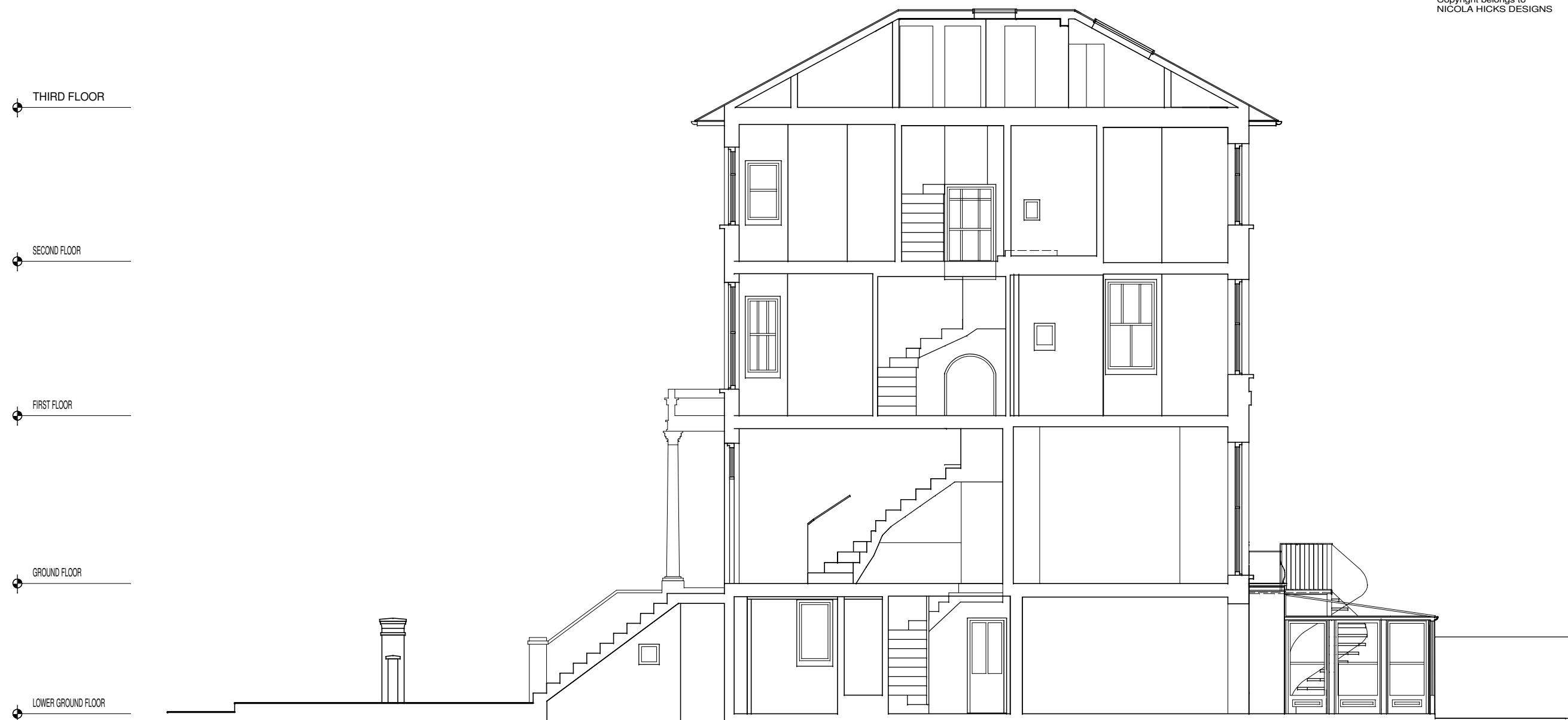
PROPOSED LONG SECTION SHOWING STAIRCASE
