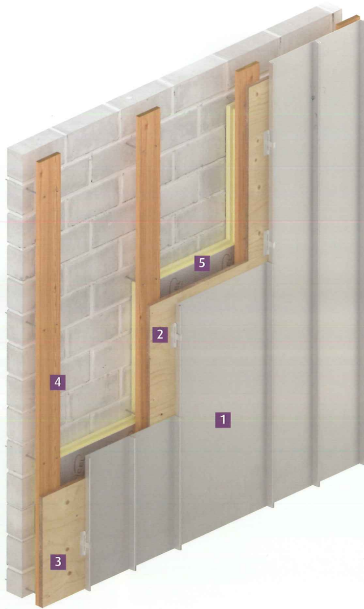
Typical standing seam panel system construction
