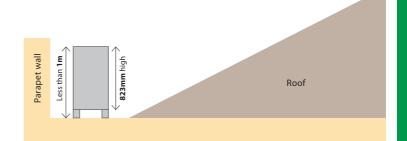
Planning issues for small commercial or residential projects in towns and cities can now be easy to overcome with a Low height version of the mini VRV range, available in 4 & 5HP with Variable Refrigerant Temperature and connection to products such as Air Curtains, Air handling units and the Emura and Nexura fan coils, the Low height Mini VRV range brings a whole new level of versatility to the VRV range.
