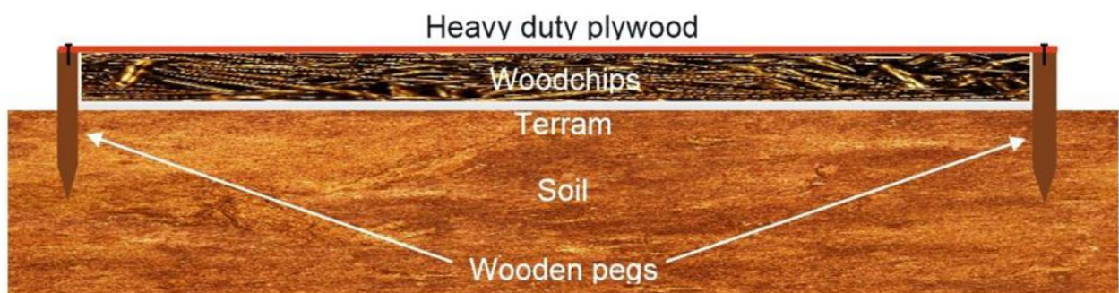
Figure 4. Specification for ground protection.
